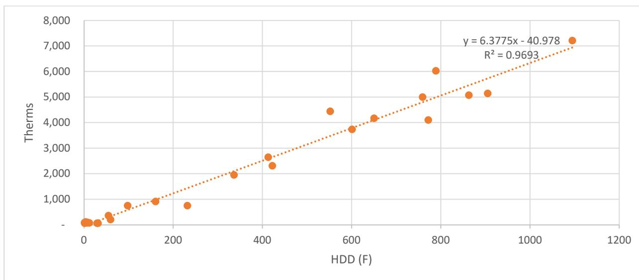
Figure 15: Regression Analysis for Natural Gas Consumption and HDD
