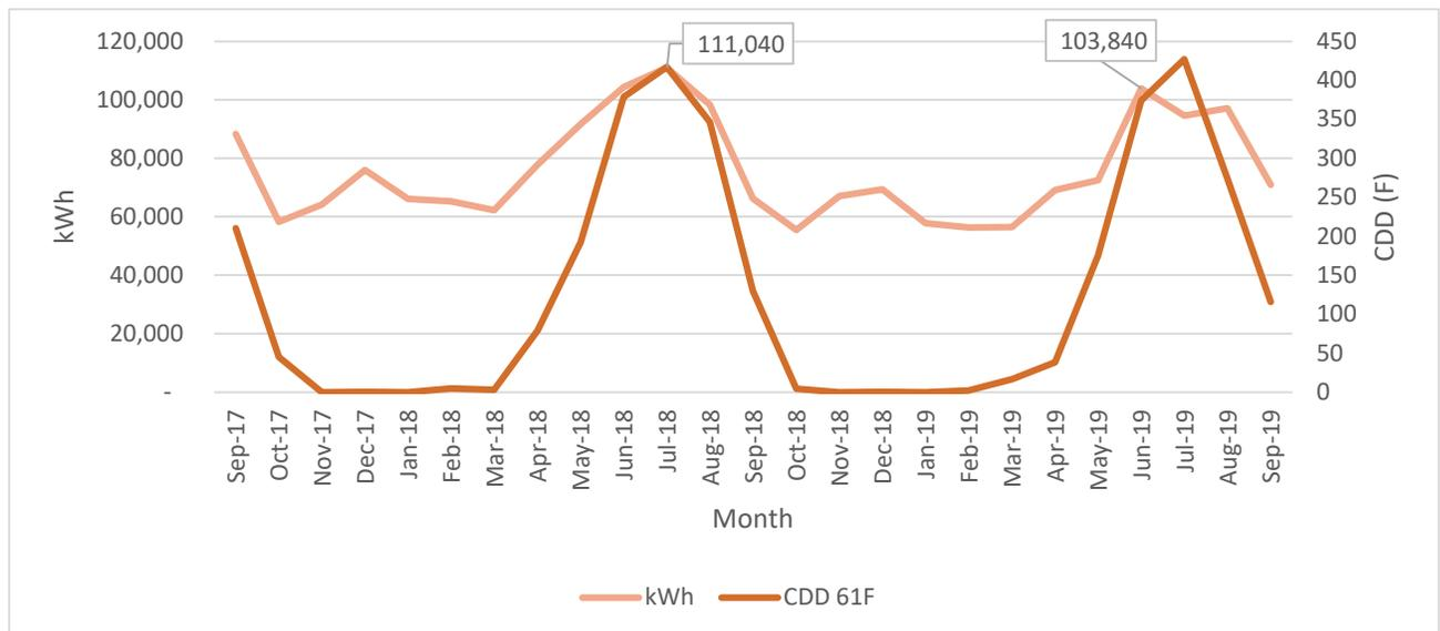
Figure 13: Past 2 Years of Electricity Consumption with CDD
