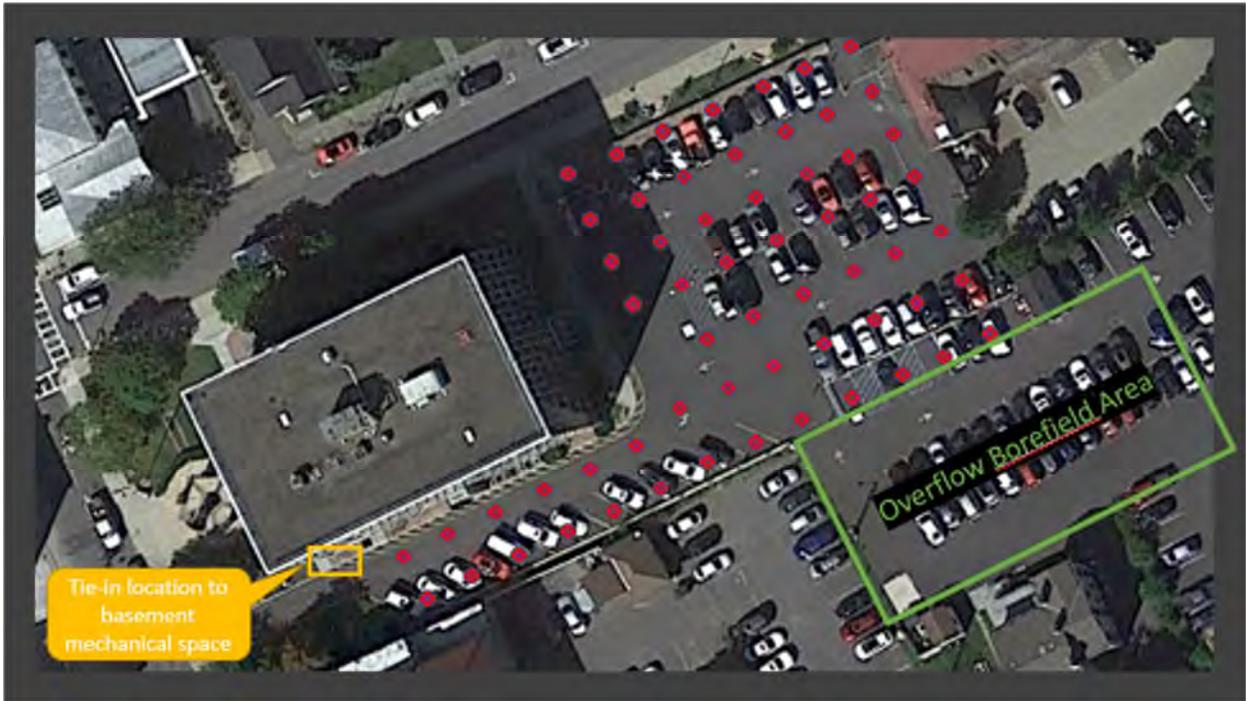
Figure 18: Heat Exchanger grid layout
