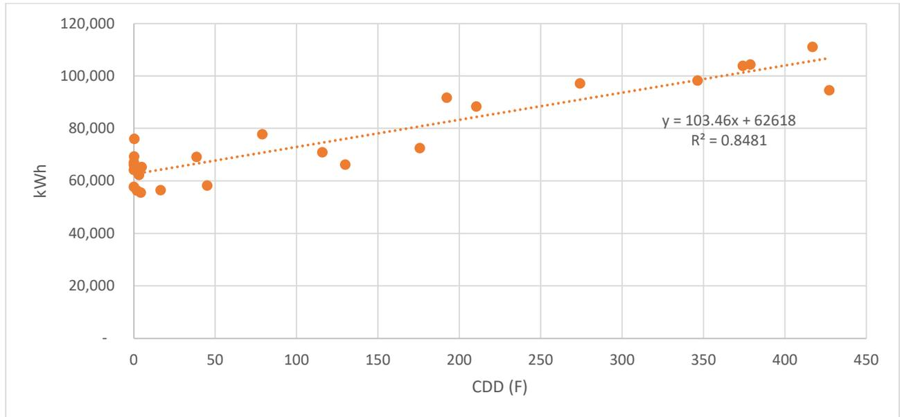
Figure 12: Regression Analysis for Electric Consumption and CDD
